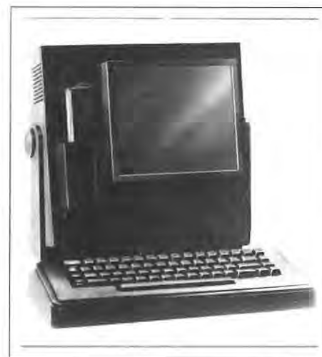
Fig. 6: Video monitor containing a 2-in.-diameter single-crystal CRT. The image from the tube is projected onto an 11-in.-diagonal screen.
