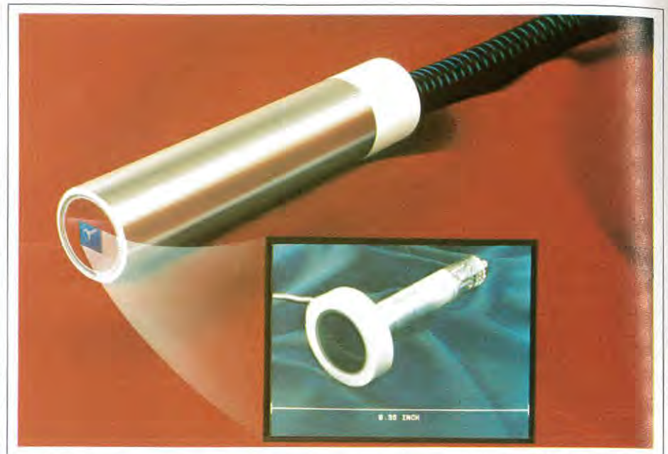
Fig. 4: A 3-in.-diameter single-crystal CRT imaged onto an AT&T Targa16 image capture board and then transferred, along with the scale, onto a 1-in.-diameter single-crystal CRT. The picture on the 1-in. tube is a standard 525-line TV raster display; resolution is approximately 1500 lines/in.
